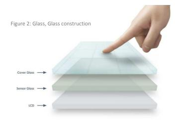
3GS is also available and used when there is a need for special cover glass materials such as Gorilla glass or polycarbonate. Glass only constructions are always better from an optical performance standpoint compared to film.
